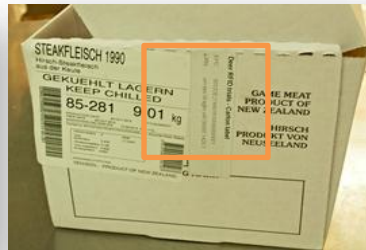
Figure 5.10 - UHF RFID tags positioned on cartons
